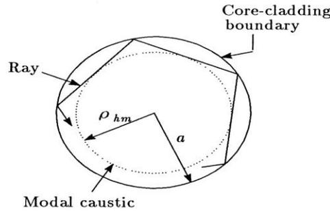
Fig. 2. Top view of the pillbox resonator with whispering gallery Modes
