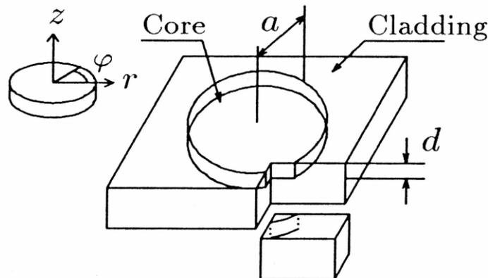
Fig. 1. Configuration of pillbox resonator
