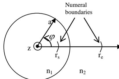
Fig. 3. Pillbox resonator showing the calculated region bounded by the numerical boundaries
