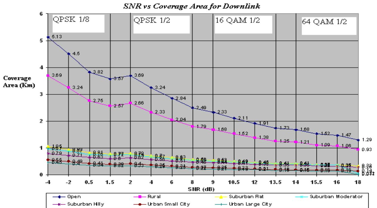
Fig. 3: Changes in coverage area for different SNR for different modulation schemes (Downlink)
