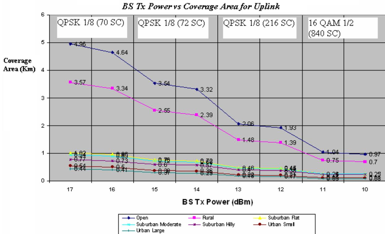
Fig. 6: Changes in Coverage Area for different BS Tx power for different modulation schemes (Uplink)
