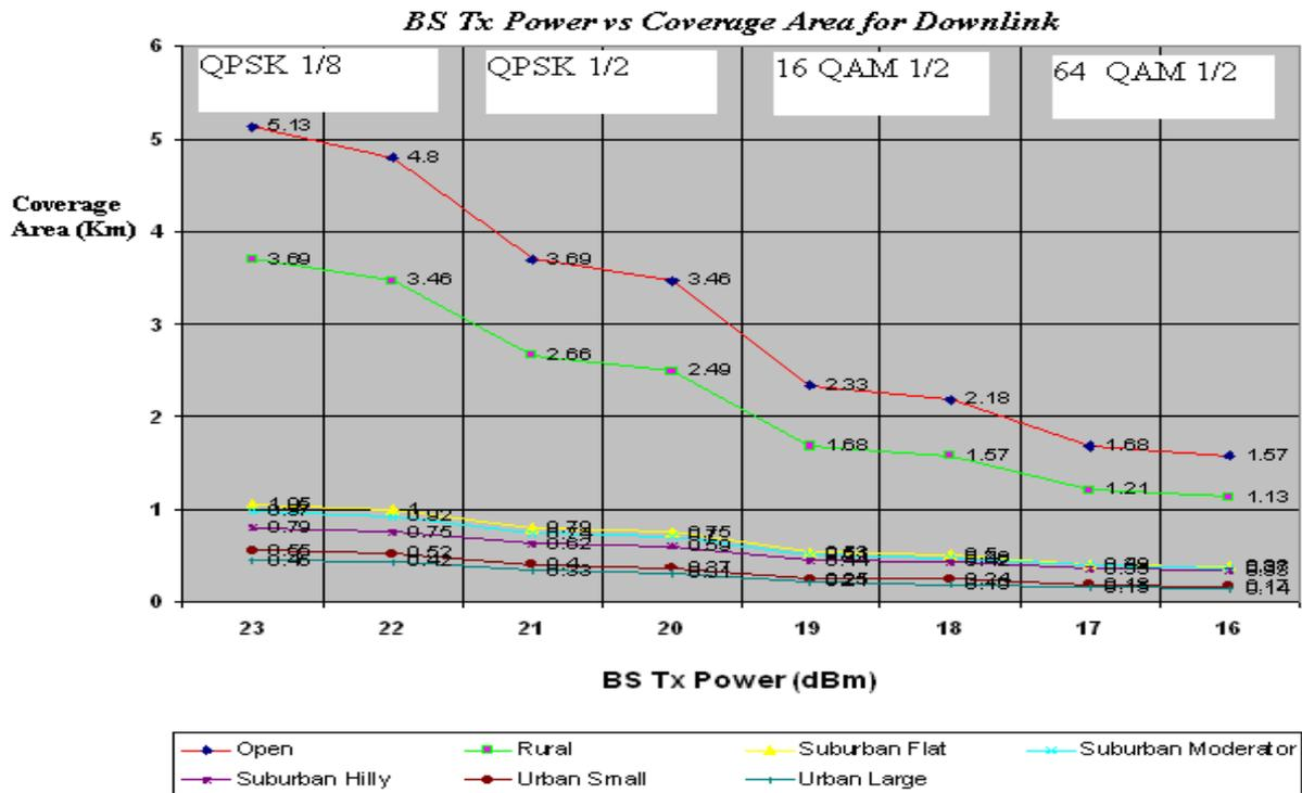
Fig. 5: Changes in coverage area for different BS Tx power for different modulation schemes (Downlink)
