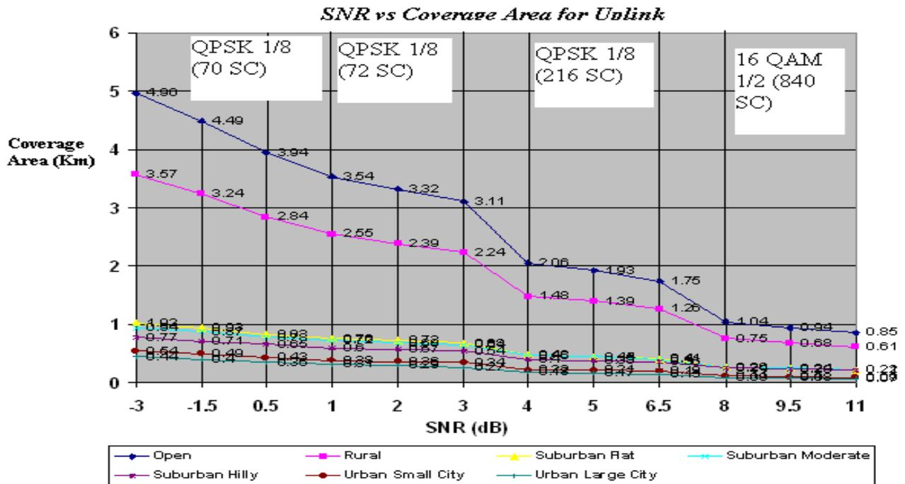
Fig. 4: Changes in coverage area for different SNR for different modulation schemes (Uplink)
