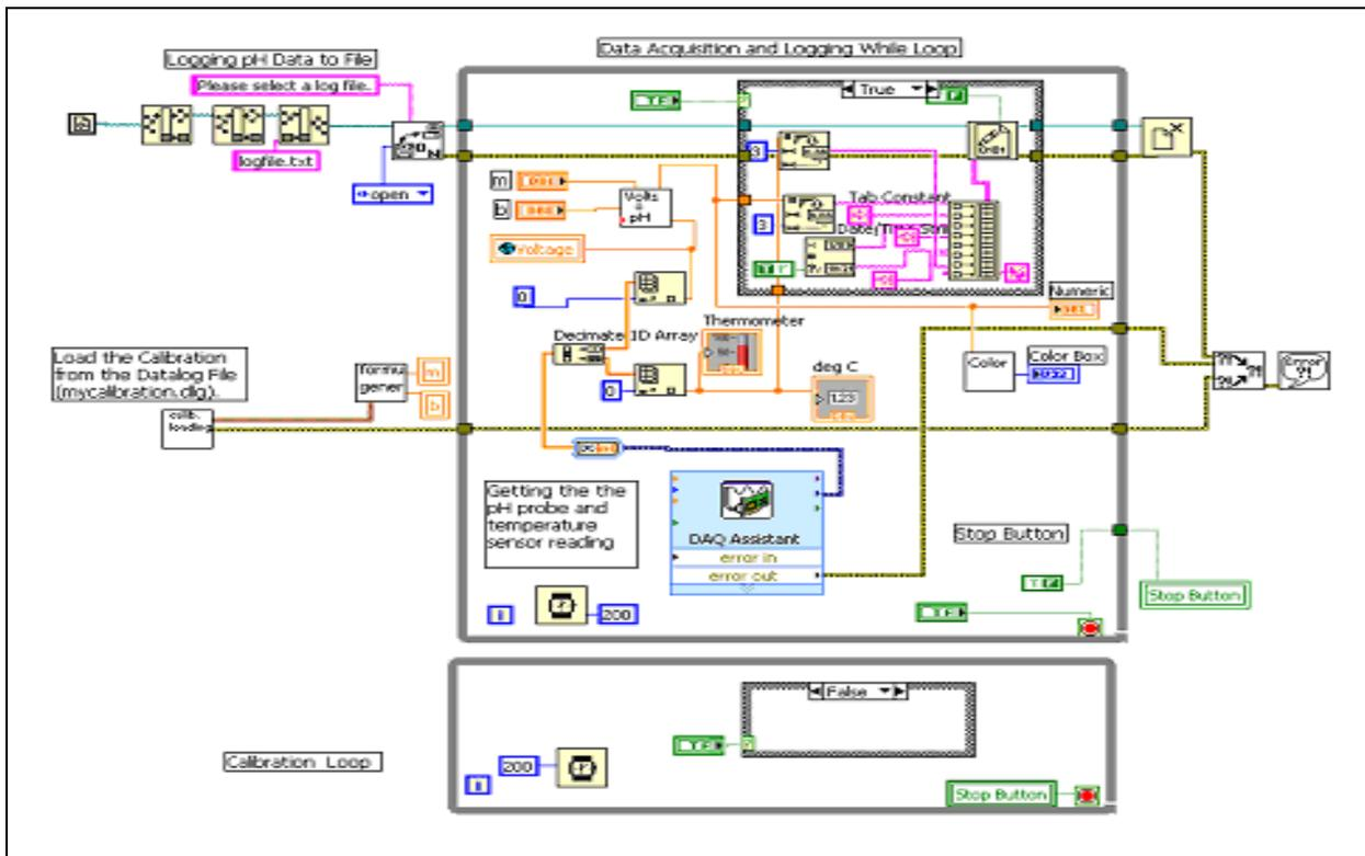
Fig. 6: Block diagram of the data acquisition system for pH and Temperature
