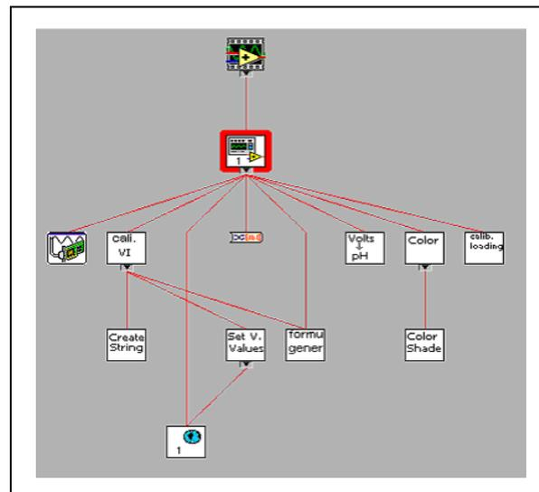
Fig. 8: VI hierarchy of the DAQ system
