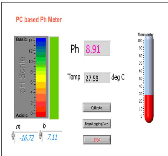
Fig. 7: User interface of the DAQ system
