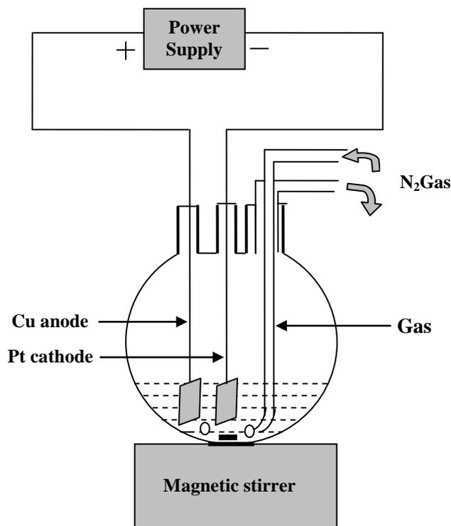
Fig. 1: Electrochemical cell for synthesis of CuO nanoparticles.
