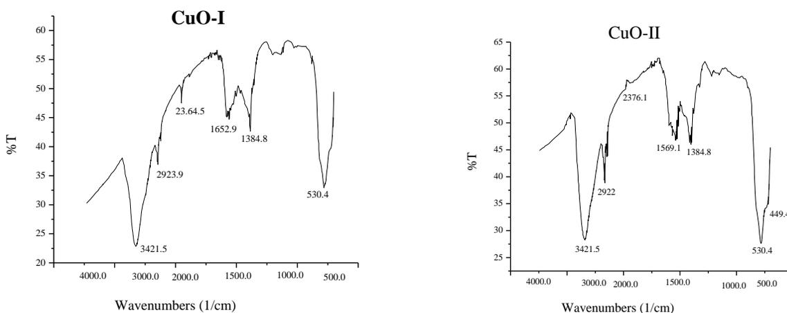
Fig. 4: Fourier transform infrared spectra of CuO-I and CuO-II nanocrystals. CuO-I sample shows 530.4, 1384.8, 1652.9, 2364.6, 3421.5 vibrational mode while CuO-II sample shows 449.4, 530.4, 1384.8, 1569.9, 2376.1, 2922, 3421.5 respectively.
