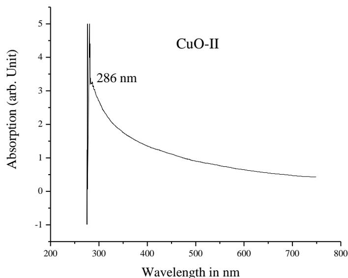
Fig. 3: Optical absorption spectra of (a) CuO-I (10nm) and (b) CuO-II(12nm) nanocrystals dispersed in acetonitrile, showing absorption feature at 300 nm and 286 nm respectively.
