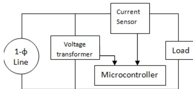
Fig. 3 Architecture of Energy Meter
