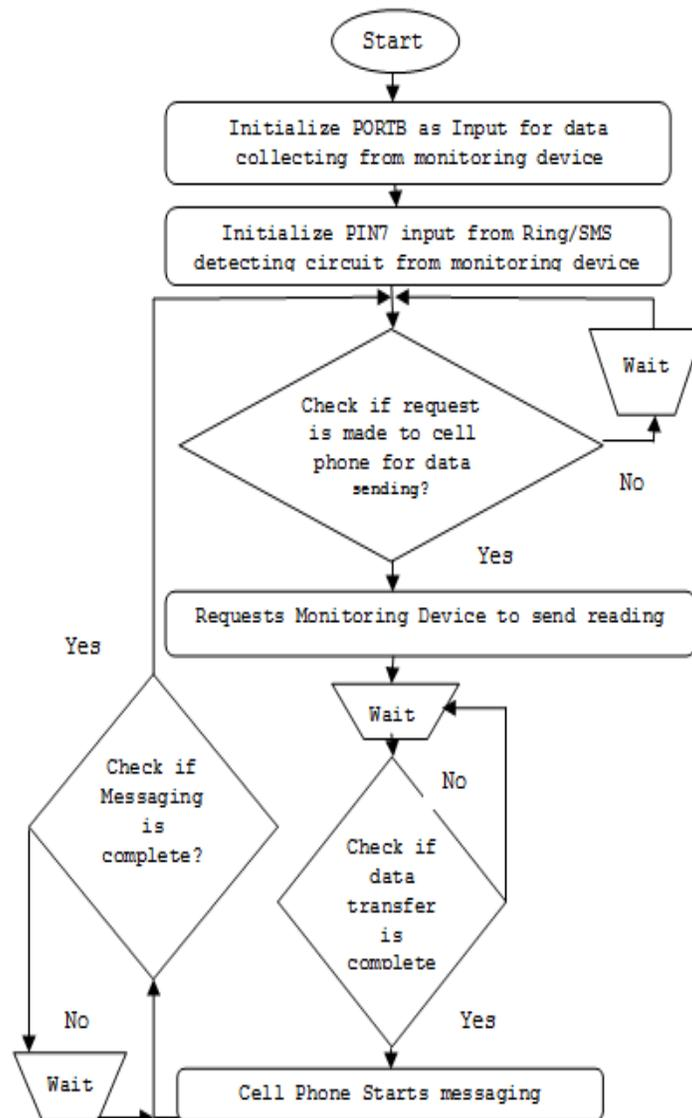
Fig.4 Flow Diagram of Microcontroller operation of Data Sending Device
