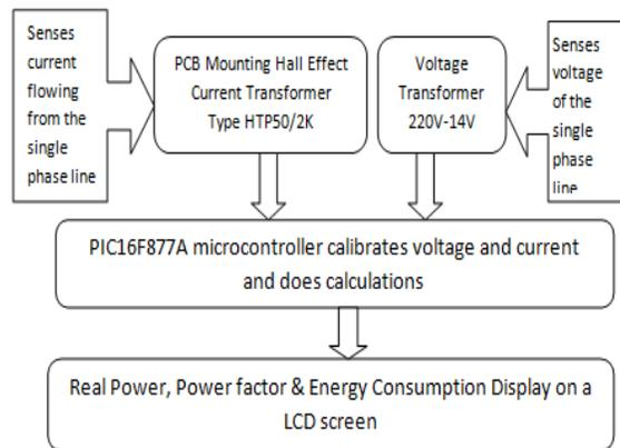
Fig. 1 Block diagram of Smart energy meter
