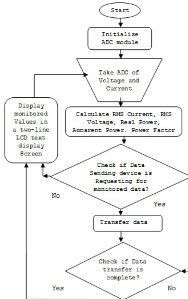
Fig.4 Flow Diagram of Microcontroller operation of Energy Meter
