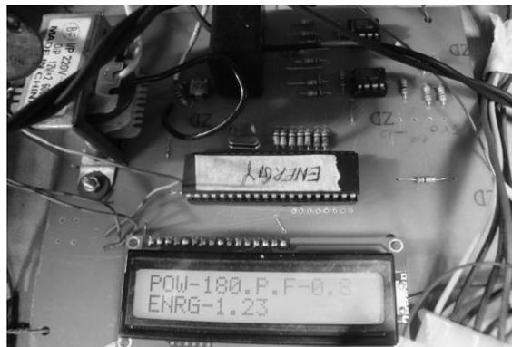
Fig.6 Displaying meter reading with a LCD display
