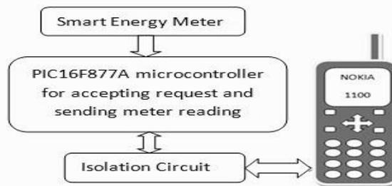
Fig. 2 Block diagram of Data Sending Device
