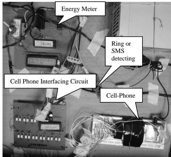
Fig.5 Combining Energy Meter with Data Sending Device
