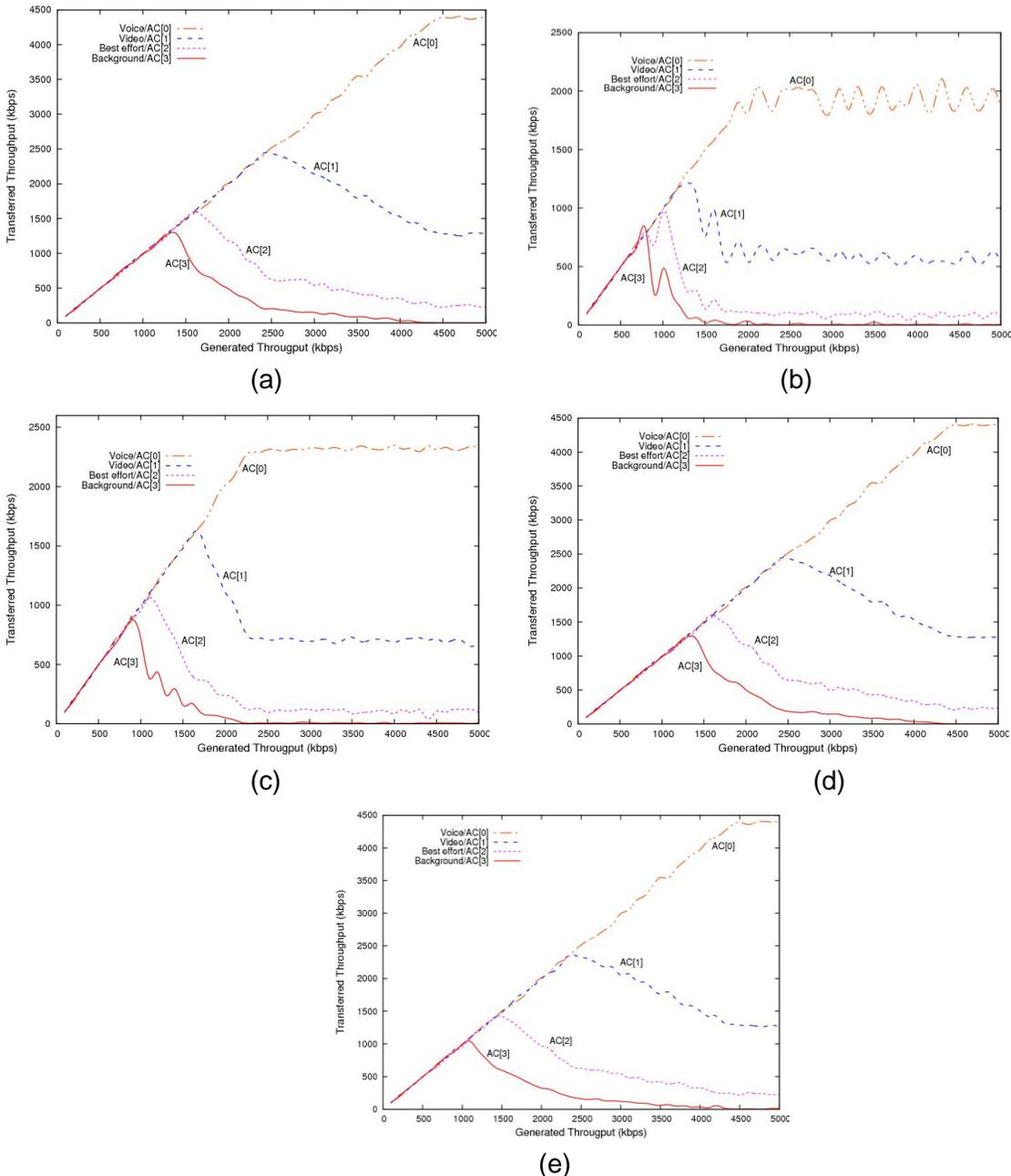
Figure 3: Generated Vs Transferred Throughput Curves of Voice, Video, Best effort and Background Traffic Access Category, observed in the simulation study with the first (a), second (b), third (c), fourth (d)
