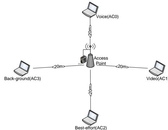
Figure 1: The AP is at the centre of the topography while client nodes are positioned at equal distances from the AP
