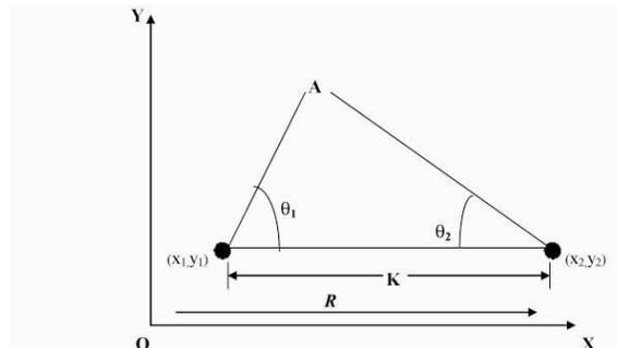
Figure 3: Determining the position of object "A" in 2 dimensions.
