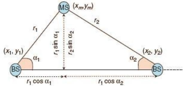
Fig. 1: combining AOA measurements
