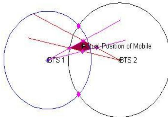
Fig. 6: Superimposing the areas from AOA angle spread and NLOS distance.
