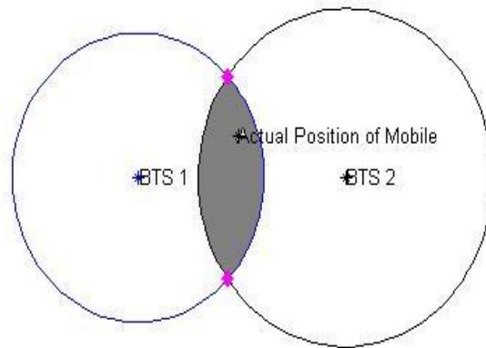
Fig. 5: overlapped area of MS location for NLOS distance
