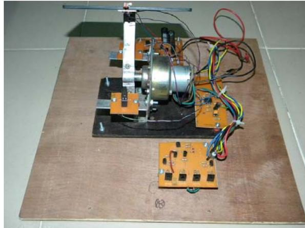
Fig 8: Tracking Device backside view
