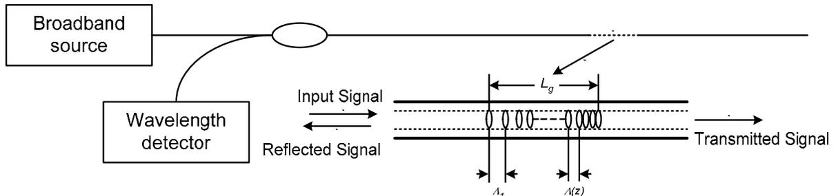
Fig. 2: LCFBG based sensor system with reflection detection.
