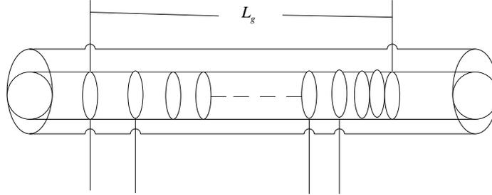
Fig. 1: Linearly chirped Bragg grating where periodicity  $\Lambda$ , varies as a function of position  $z$ .
