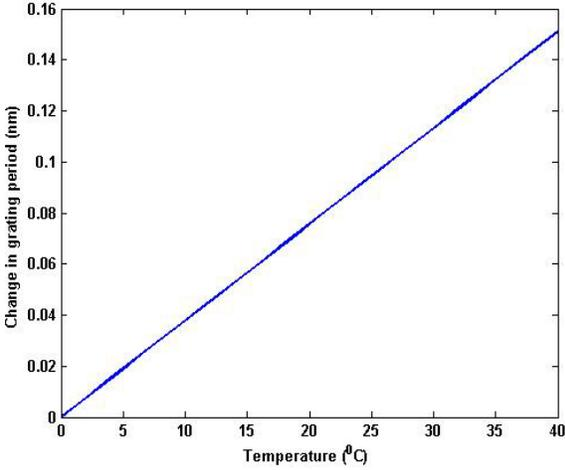
Fig. 5: Change in grating period as a function of temperature.
