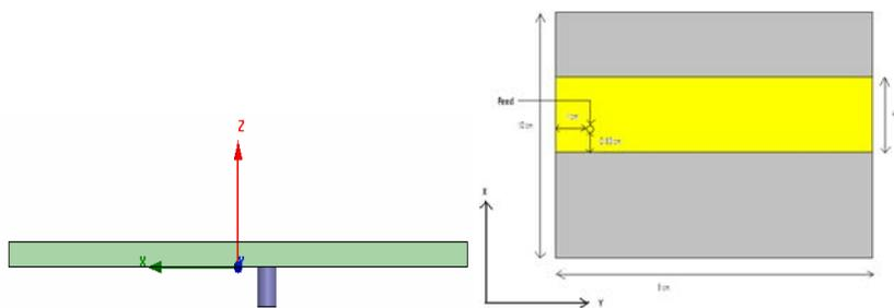
Fig. 1: (a) Proposed antenna (side view) (b) top view
