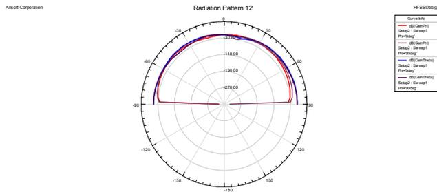
Fig. 4: Radiation Pattern of the antenna at 4 GHz
