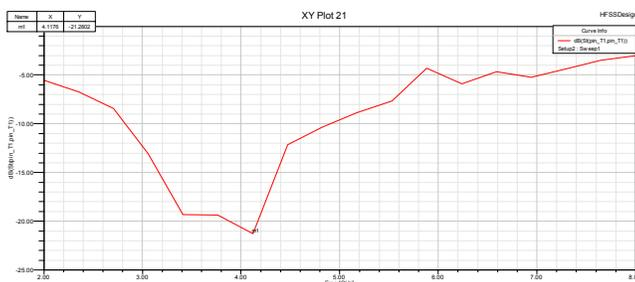
Fig. 2: Return loss of proposed design
