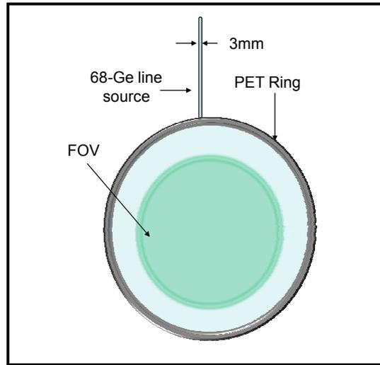
Fig. 1: Block diagram for the measurement of PET sensitivity; the 68-Ge line source was placed at the axial position of the camera field-of-view.
